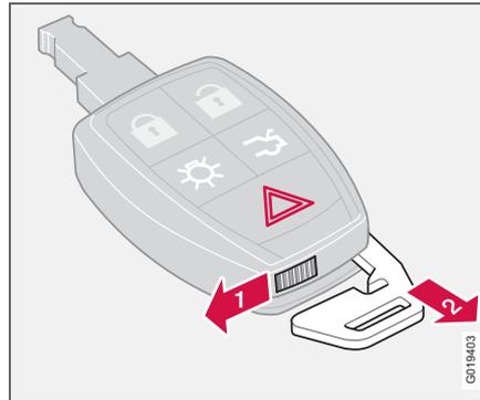
Using the remote control's detachable key blade:
