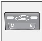
Recirculation can be used to shut out bad air, exhaust fumes, etc. from the passenger compartment. The air in the passenger compartment is recirculated, i.e. no
