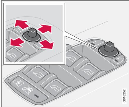
The controls for adjusting the two door mirrors are at the front of the driver's door armrest. The rearview mirrors can be operated in ignition position **I** and **II**.
