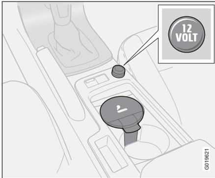
The electrical socket can be used for 12 V accessories, such as mobile phone chargers and coolers. The maximum current is 10 A. For the socket to supply current, the ignition key must be in at least position I.
