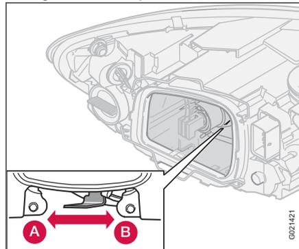
The headlamp control should be in position (A) for left-hand traffic and position (B) for right-hand traffic.
