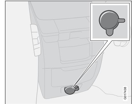
The electrical socket can be used for various accessories, such as mobile phone chargers and coolers.
