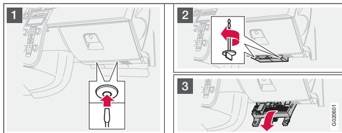
The fuse box has 50 fuse positions. The fuses are located under the glovebox. The box also provides space for several spare fuses. Tools for fuse replacement are located in the relay/fuse box in the engine compartment, see page 200.
