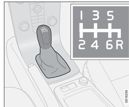
Depress the clutch pedal fully with each gear change. Remove your foot from the clutch pedal between gear changes! Follow the appropriate shifting pattern.
