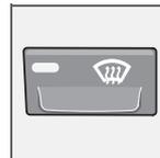
Quickly removes misting and ice from the windscreen and side windows. Air flows to the windows at high fan speed. The light in the defroster button illuminates
