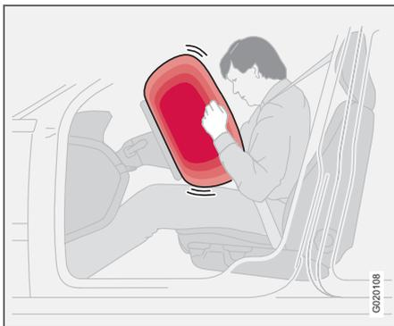
The car has an SRS airbag (Supplemental Restraint System) to supplement the protection afforded by the seatbelt on the driver's side. This airbag is folded up into the centre of the steering wheel. The steering wheel is marked **SRS AIRBAG**.
