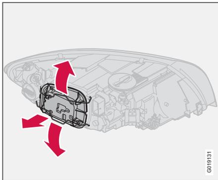
**Removing the cover and bulb:**
