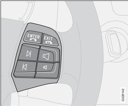
The four buttons at the bottom of the steering wheel keypad control the radio and the phone. The function of a button depends on which system is active. The steering wheel keypad can be used to scroll between preset stations, change CD tracks and adjust the volume.
