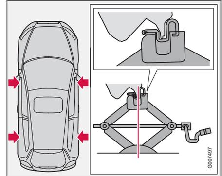
Set up the warning triangle if a wheel must be replaced at a busy location. Make sure that the car and jack are on a firm horizontal surface.
