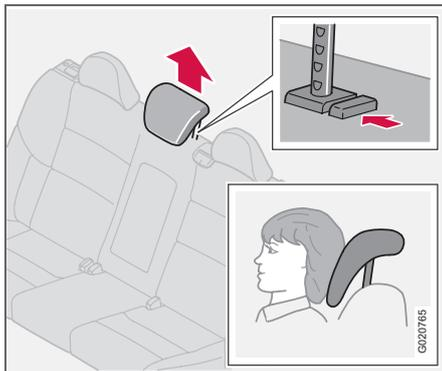
All head restraints can be adjusted vertically to suit the height of the passenger. The upper edge of the head restraint should be aligned with middle of the back of the head. Raise the head restraint as necessary. To lower the head restraint, press the button by the right-hand pillar at the same time as pushing down the head restraint. To remove the head restraint, press the button by the right-hand pillar while lifting out the head restraint.
