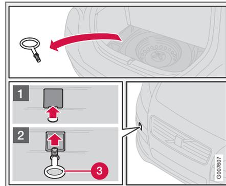
Use the towing eye if the car needs to be towed on the road. The towing eye is attached in the recess on the right-hand side of the front or rear bumper.
