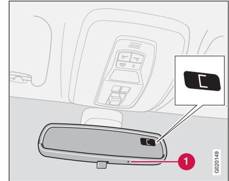
The earth is divided into 15 magnetic zones. The compass is set for the geographical area to which the car was delivered. The compass should be calibrated if the car is moved across several magnetic zones.
