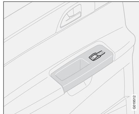
The rear door windows can be operated with the control on each door or with the switch on the driver's door. If the light in the switch for blocking the rear power windows (located in the control panel in the driver's door) is illuminated, the rear door windows can only be operated from the driver's door. The windows in the rear doors are operated in the same way as the windows in the front doors.
