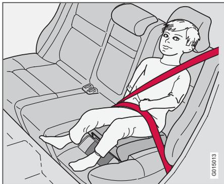
Volvo's integrated booster cushion for the outer rear seats is specially designed to provide optimum safety for children. Combined with the regular seatbelts, the booster cushion is approved for children weighing between 15 and 36 kg.
