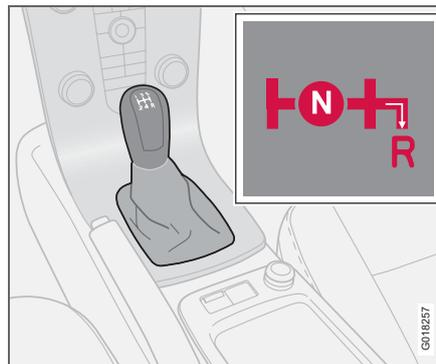
Only engage reverse gear when the car is stationary. To engage reverse gear, the gear lever must first be put in position **N**. Reverse gear cannot therefore be engaged directly from fifth gear due to the reverse gear inhibitor.
