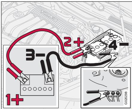
If the battery in the car has become flat, you can "borrow" electric current from either a separate battery or the battery in another car. Always make sure the crocodile clips on the jump leads are attached securely to eliminate sparks during the start attempt.
