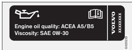
When the oil decal shown alongside here is in the car's engine compartment, the following applies. See location on page 232.
