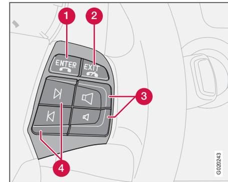
When the phone is active, the steering wheel keypad is locked to phone functions. To control the audio system, the phone must be in standby mode.
