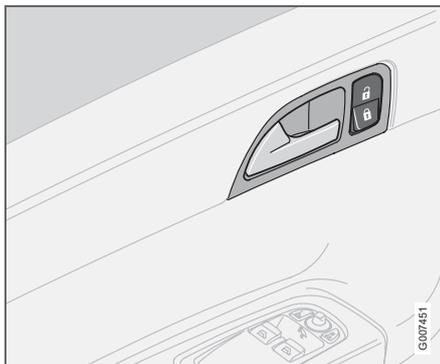
The doors and the boot lid can be locked or unlocked simultaneously using the lock button by the door handle.
