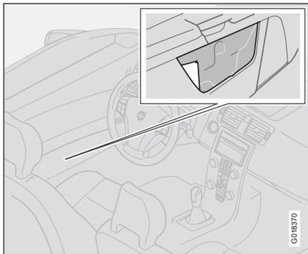
In the front door storage compartments, in the rear section, is an integrated holder for an ice scraper. Insert the ice scraper into the holder. The ice scraper must be the type with a rectangular plastic section, approx. 3 mm thick. In front of the ice scraper is a space for a soda can.
