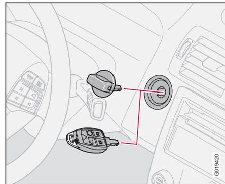
If the remote control battery is discharged then the Keyless Drive function does not work. In which case, start the car by using the remote control as ignition dial.
