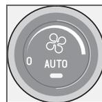
The **AUTO** function automatically regulates climate control and maintains the selected temperature. The AUTO function controls heating, air conditioning, fan speed, recirculation, and air distribution. If you select one or more manual functions, the other functions continue to be controlled automatically. All manual settings are switched off when **AUTO** is switched on. The display shows **AUTO CLIMATE**.
