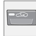
Recirculation can be used to shut out bad air, exhaust fumes, etc. from the passenger compartment. The air in the passenger compartment is recirculated. No outside air is taken into the car when this function is activated. Recirculation (together with the air conditioning system) cools the passenger compartment more quickly in hot weather. If the air in the car recirculates for too long, there is a risk of the windows misting.
