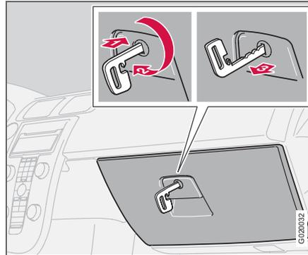
This function is intended for when the car is left for service, with a hotel parking valet or similar. The glovebox is then locked and the boot lid lock is disconnected from the central locking. The cargo area cannot be opened with either the central locking button in the front doors or the remote control.
