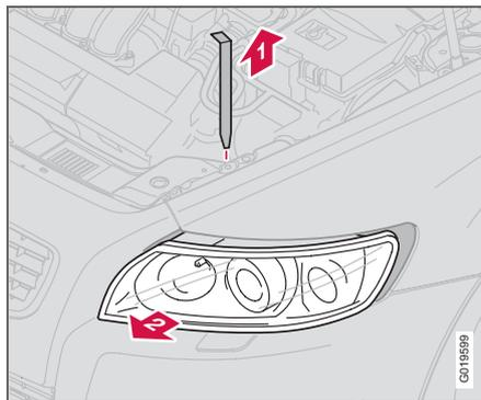
All front bulbs (except for fog lamps) are changed by first removing the lamp housing from the engine compartment.
