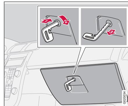
The glovebox can only be locked/unlocked using the remote control's detachable key blade. For information on removing the key blade, see page 99.
