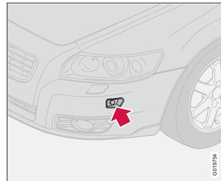
Connecting the engine block heater
