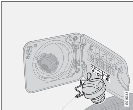
Switch off the fuel-driven heater before refuelling.
