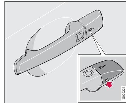
If central locking cannot be activated with the remote control, e.g. if the batteries are discharged, then the driver's door can be opened as follows:
