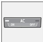
**ON:** Air conditioning is on. It is controlled by the system's AUTO function. This way, incoming air is cooled and dehumidified.
