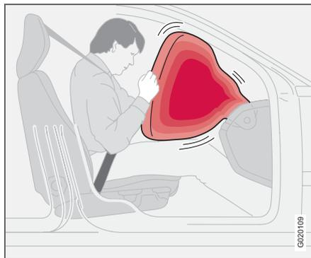
The car has an airbag<sup>1</sup> to supplement the protection afforded by the seatbelt on the passenger side. This airbag is folded up into a compartment above the glovebox, and its cover panel is marked **SRS AIRBAG**.
