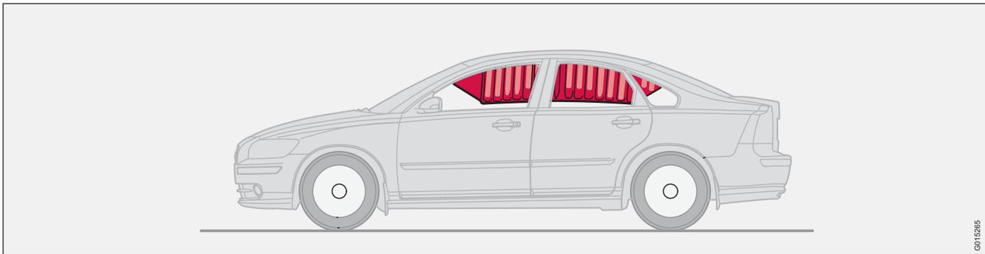
The inflatable curtain IC (Inflatable Curtain) is a supplement to the SIPS and the airbags. It is fitted in the headlining along both sides of the roof and protects all of the vehicle's outer seats. A sufficiently violent collision trips the sensors and the inflatable curtain is inflated. The inflatable curtain helps to prevent the driver and passengers from striking their heads on the inside of the car during a collision.
