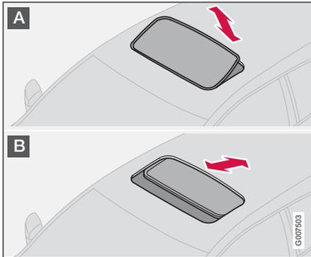
The sunroof controls are located in the roof panel. The sunroof can be opened to two positions:
