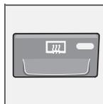
Use the defroster to quickly remove misting and ice from the rear window and door mirrors. The rear window and door mirrors are defrosted simultaneously if
