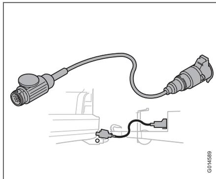
An adapter is required if the car's towbar has 13 pin electrics and the trailer has 7 pin electrics. Use an adapter cable approved by Volvo. Make sure the cable does not drag on the ground.
