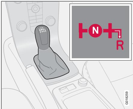
Only engage reverse gear when the car is stationary.
