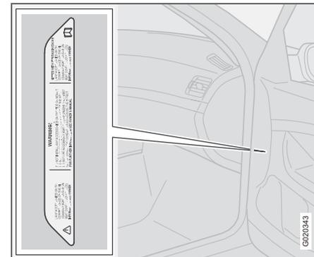
*Location of airbag decal in door opening on front passenger side in left-hand drive cars.*
