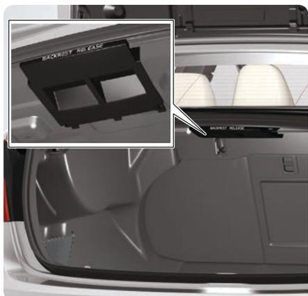
The two-section backrest can be folded forward – both sections together or separately.
