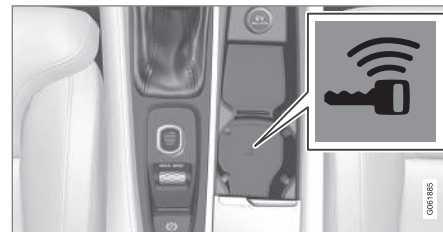
Backup reader's location in the tunnel console.
