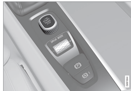
Start knob in the tunnel console.
