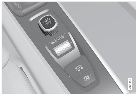
Start knob in the tunnel console.
