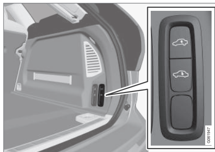
Controls for raising/lowering the rear end of the vehicle.
