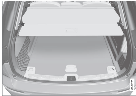
Cargo cover in full-cover position.
