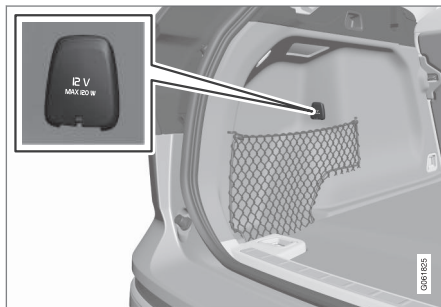
12 V electrical socket in cargo area*.
