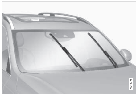
Wiper blades in service position.
