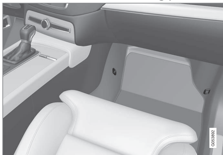
Mounting point locations in the front seat.
