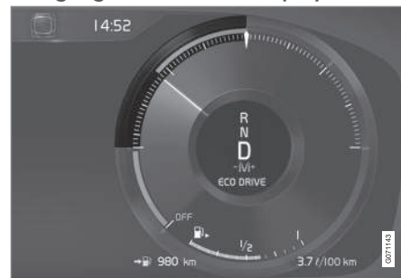
Eco gauge in the 12-inch driver display*.
