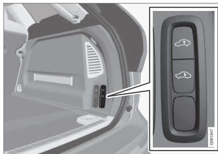
Controls for raising/lowering the car's rear section.
