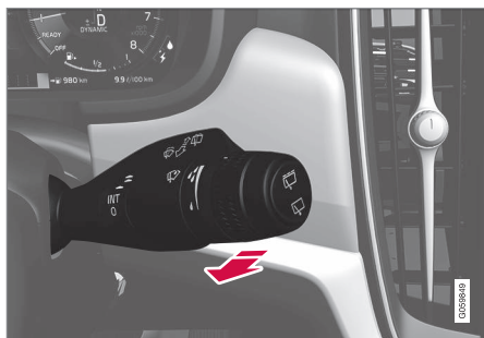
Washing function, right-hand stalk switch.
