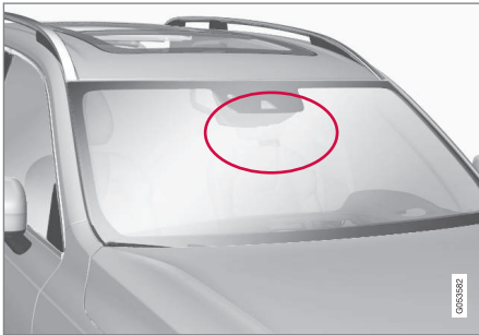
Radar unit location
