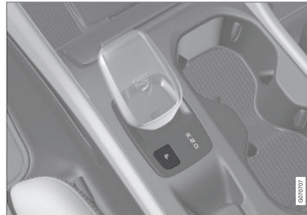
Overview of gear selector and gear position P for the small gear selector.
