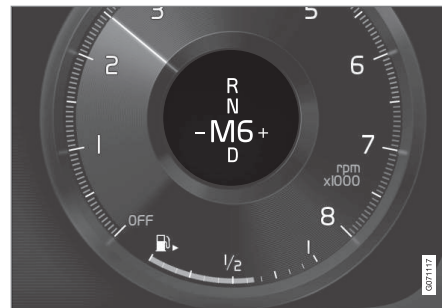
Overview of gear shift pattern in the instrument panel for the small gear selector.
