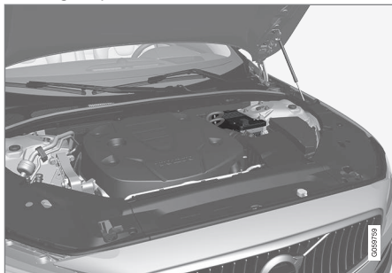
The 12 V support battery is located in a box next to the strut tower.
