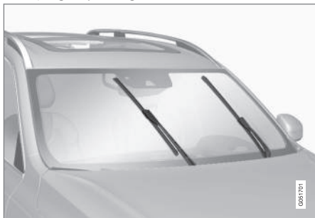
Windshield wipers in the service position.
