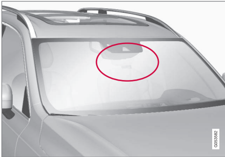
Location of radar sensor
