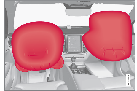
Driver/passenger side front airbags.
