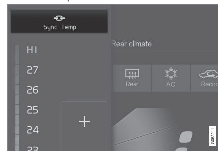
Synchronization button on the driver's side temperature control.
