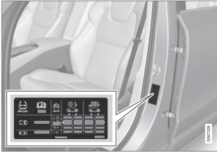
Location of the tire pressure placard
