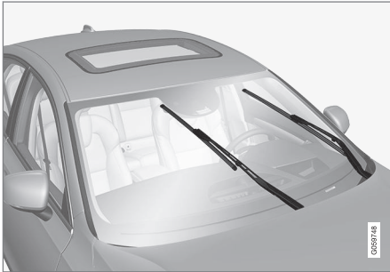
Viskerblader i servicestilling.
