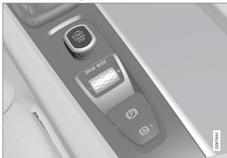
Start knob in the tunnel console.
