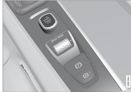
Start knob in the tunnel console.
