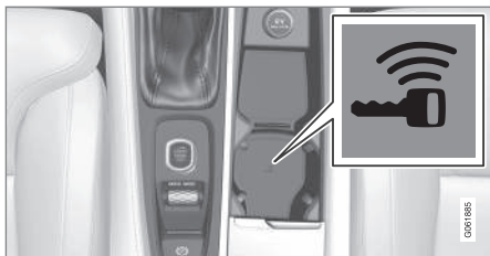
Location of the backup reader in the tunnel console.
