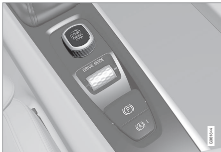
Start knob in the tunnel console.
