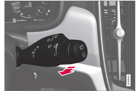
Washing function, right-hand stalk switch.
