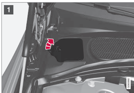
Coolant expansion tank.
