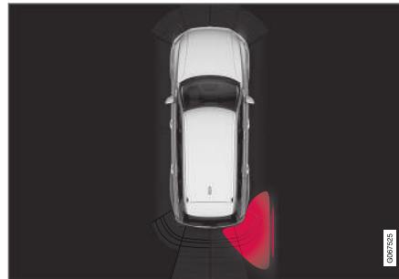
Illuminated icon for CTA in the Park Assist System graphic on the screen.
