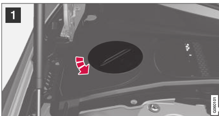
Coolant expansion tank, left-hand drive car.
