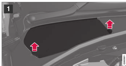
Coolant expansion tank, right-hand drive car.
