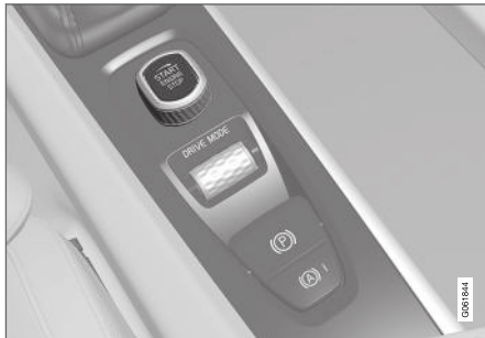
Start knob in the tunnel console.
