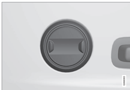
Control in cars with two-way lumbar support*.
