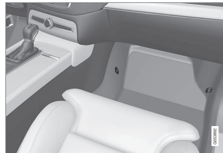
Mounting point locations in the front seat.
