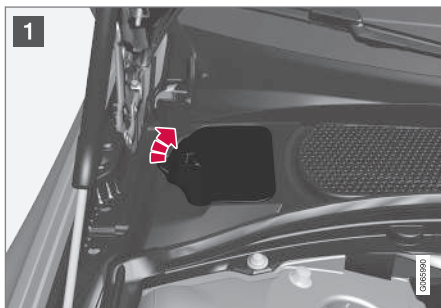
Coolant expansion tank.
