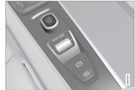
Start knob in the tunnel console.
