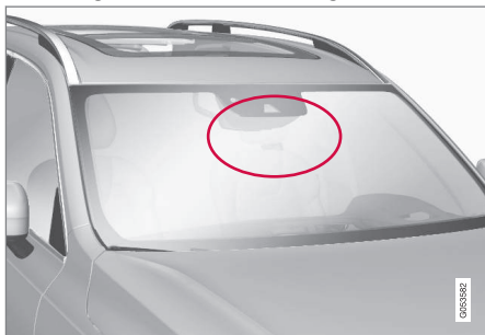
Location of the camera unit.
