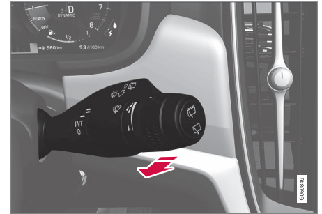
Washing function, right-hand stalk switch.
