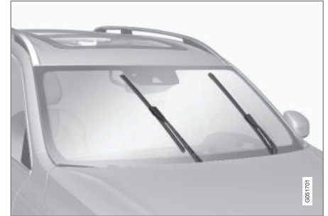
Wiper blades in service position.
