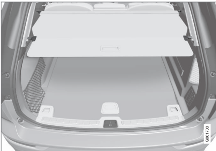
Cargo cover in full-cover position.
