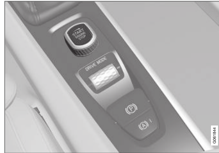
Start knob in the tunnel console.
