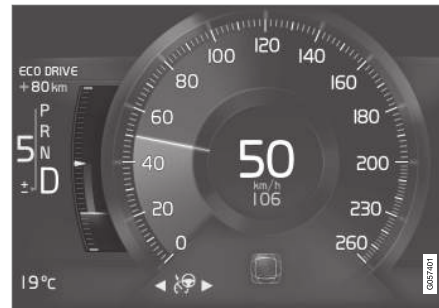
Eco gauge in the 8-inch driver display.
