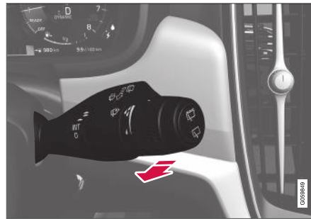
Washing function, right-hand stalk switch.
