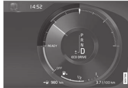
Eco gauge in the 12-inch driver display*.
