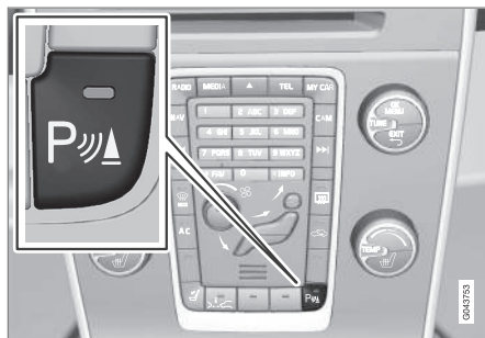
On/Off for parking assistance and CTA sensors.
