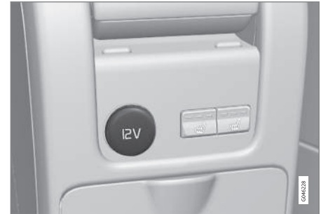
12 V socket in tunnel console, rear seat.
