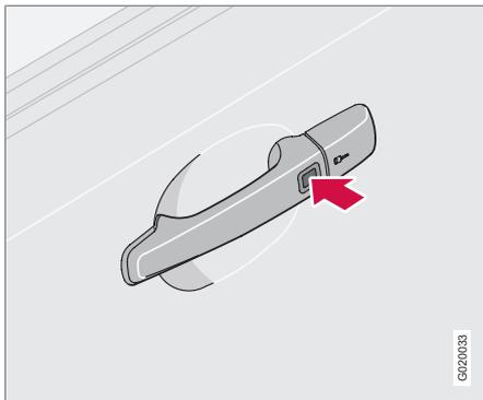
Cars with the keyless system have a button on the outside door handles.
