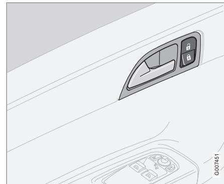
With the central locking button on the driver's door, the doors and boot lid can be locked or unlocked simultaneously.
