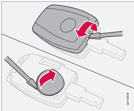
If the locks repeatedly fail to respond to signals from the remote control key at a normal distance, the battery should be replaced (type CR 2450, 3 V).
