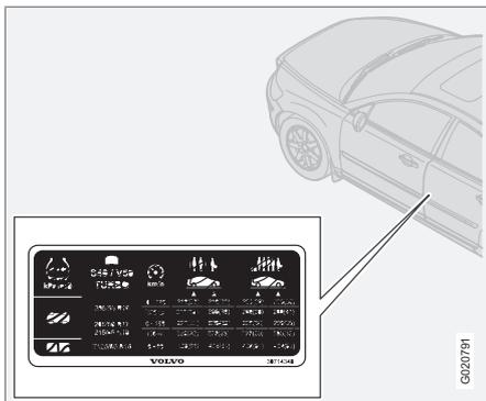
The tyre pressure label on the driver's side door pillar shows which pressures the tyres should have at different load and speed conditions.
