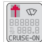
The driver is assisted by an indicator which notifies the driver when it is most advantageous to engage the next higher or lower gear - GSI (Gear Shift Indicator).
