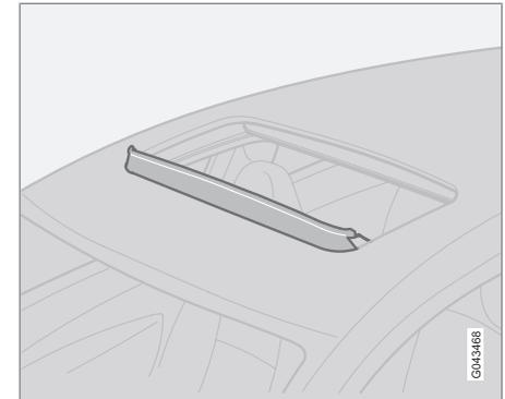
The sunroof has a wind deflector that is folded up when the sunroof is in the open position.
