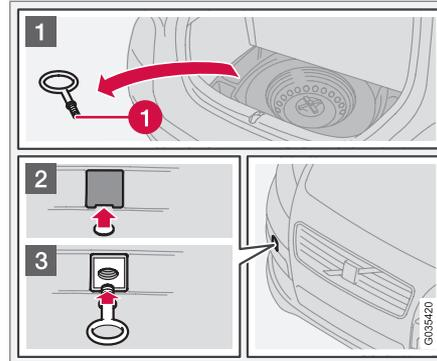
The towing eye is screwed into a threaded socket behind a cover on the right-hand side of the bumper, front or rear.
