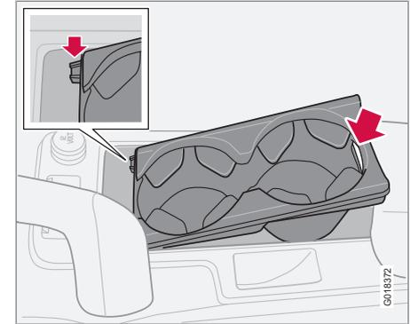
There is space for a double cup holder under the roller cover. The space can be used for storage by lifting out the cup holder. Lift at the rear edge of the cup holder where there is a recess.
