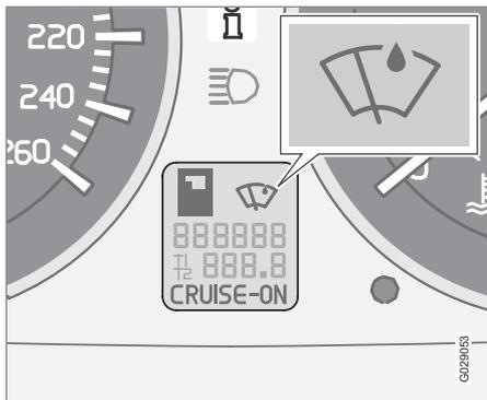
The rain sensor automatically activates the windscreen wipers based on how much water it detects on the windscreen. The sensitivity of the rain sensor can be adjusted using the thumbwheel (C), see page 67.
