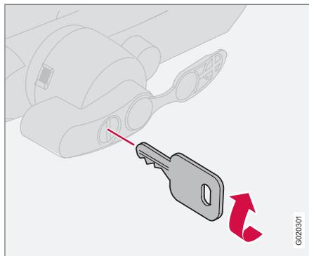
1. Insert the key and turn it clockwise to the unlocked position.
