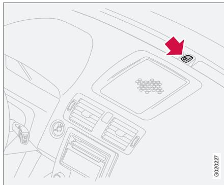
A red LED on the top of the instrument panel indicates the alarm system's status:
