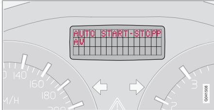
The information display shows here that the Start/Stop function has been disengaged.
