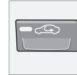
Recirculation can be used to shut out bad air, exhaust fumes, etc. from the passenger compartment. The air in the passenger compartment is recirculated. No outside air is taken into the car. Recirculation (together with the air conditioning system) cools the passenger compartment more quickly in hot weather. If the air in the car recirculates for too long then there is a risk of the windows misting.
