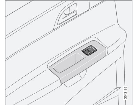
The rear door windows can be operated with the control on each door or with the switch on the driver's door. If the light in the switch for blocking the rear power windows (located in the control panel in the driver's door) is lit, the rear door windows can only be operated from the driver's door. The windows in the rear doors are operated in the same way as the windows in the front doors.
