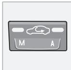
The function is selected to shut out bad air, exhaust gases etc. from the passenger compartment. The air in the passenger compartment is recirculated, i.e. no outside air is taken into the car when
