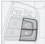
Call volume is regulated with the steering wheel keypad.
