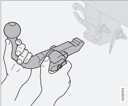
3. Turn the locking wheel down fully, until it comes to a stop. Hold it in this position while pulling the towbar rearward and upward.
