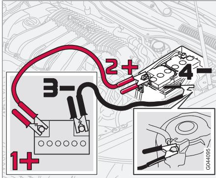
If the battery is flat then the car can be started with current from another battery.
