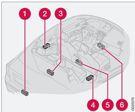
The keyless system has a number of integrated antennae located around the car:
