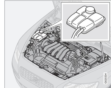
When topping up the coolant, follow the instructions on the packaging. It is important that the mixture of coolant concentrate and water is correct for the prevailing weather conditions. Never top up with water only. The risk
