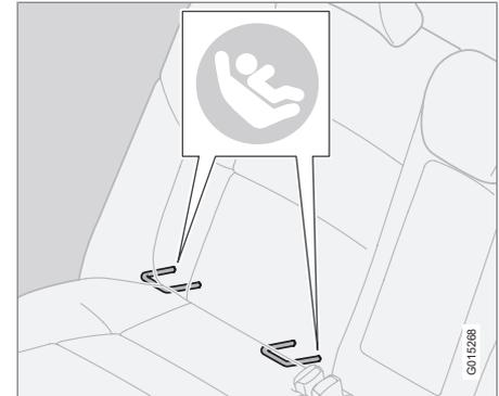
Mounting points for the ISOFIX fixture system are concealed behind the lower section of the rear seat backrest, in the outer seats.
