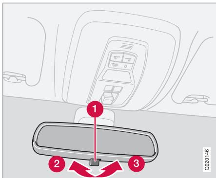
Bright light from behind could be reflected in the rearview mirror and dazzle the driver. Use dimming when disturbed by light from behind.
