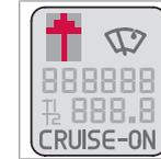
GSI - Gear Shift Indicator - advises the driver of the optimum time to change gear. The indication is given with an arrow for up and down shifting respectively in the lower information display of the combined instrument panel, see page 51.
