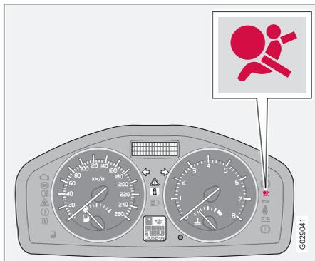
The warning symbol in the combined instrument panel illuminates when the remote control key is turned to key position **I**, **II** or **III**. The symbol goes out after approx. 6 seconds provided the airbag system is fault-free.
