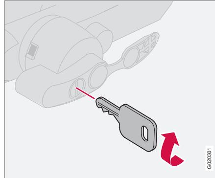
2. Ensure that the mechanism is in the unlocked position by turning the key clockwise.
