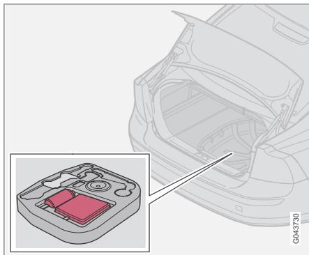
The emergency puncture repair kit is used to seal a puncture as well as to check and adjust the tyre pressure. It consists of a compressor and a bottle with sealing fluid. The kit works as a temporary repair. The sealing fluid bottle must be replaced before its expiration date and after use.
