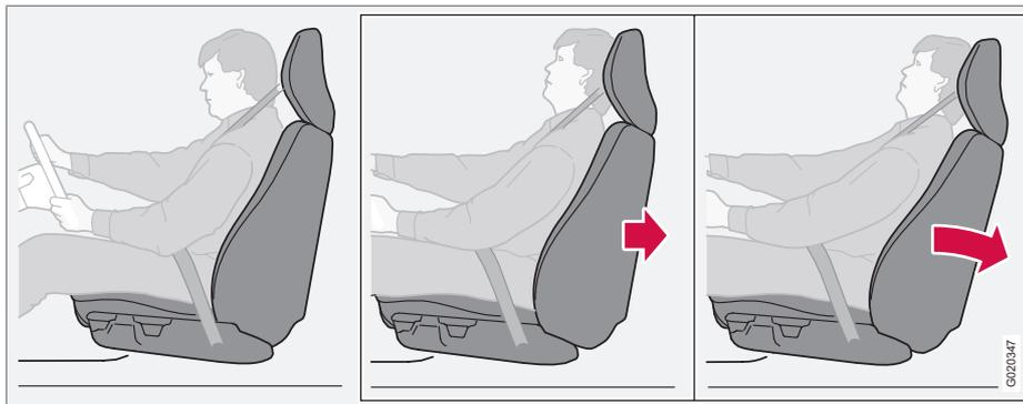
The whiplash protection system (WHIPS) consists of energy absorbing backrests and specially designed head restraints for the front seats. The system is actuated by a rear-end collision, where the angle and speed of the collision, and the nature of the colliding vehicle all have an influence.
