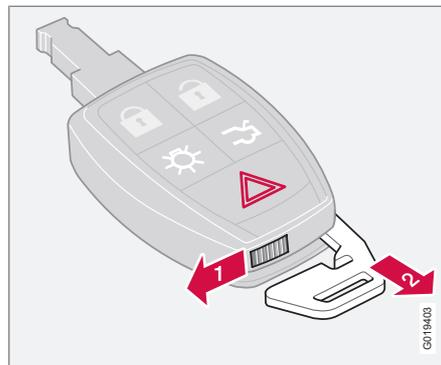
Using the remote control key's detachable key blade:
