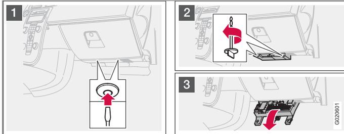
The fuse box has 50 fuse positions. The fuses are located under the glovebox. The box also provides space for several spare fuses. Tools for fuse replacement are located in the relay/fuse box in the engine compartment, see page 236.
