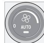
Turn the knob to increase or decrease fan speed. If **AUTO** is selected then fan speed is regulated automatically. The previously set fan speed is disengaged.
