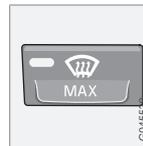
Used to quickly remove misting and ice from the wind-screen and side windows. Air flows to the windows at high fan speed. The light in the defroster button illuminates when the function is active.
