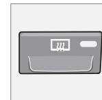
Heating is used to quickly remove misting and ice from the rear window and door mirrors. Press the button once to start simultaneous rear window and rearview mirror defrosting. The function is
