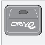
In certain situations, it may be advisable to temporarily switch off the automatic Start/Stop function - this is carried out by pressing this button once, at which point the button's lamp goes out.
