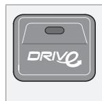
The display text **ENGINE IN AUTO START**, and the button's illuminated green lamp, reminds - and indicates - that the engine has been auto-stopped.
