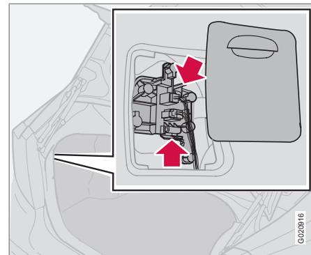
All bulbs in the rear lamp cluster are replaced from inside the cargo area.
