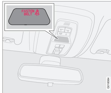
Unbelted occupants will be reminded to fasten their seatbelts by means of an audio and visual reminder. The audio reminder is speed dependent, and in some cases time dependent. The visual reminder is located in the roof console and the combined instrument panel.
