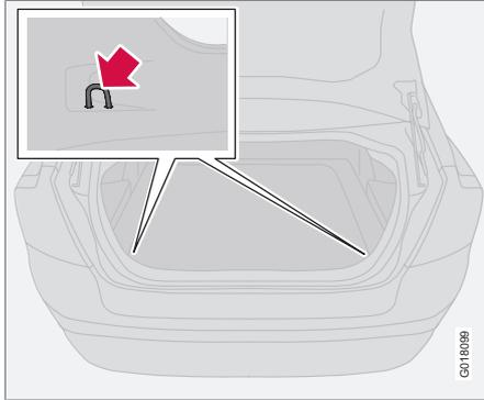
The load retaining eyelets are used to fasten straps or nets to anchor items in the cargo area.
