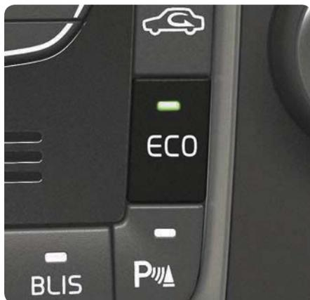
On press on **ECO** activates an optimal fuel-efficient driving program including, amongst other things, the following changes:
