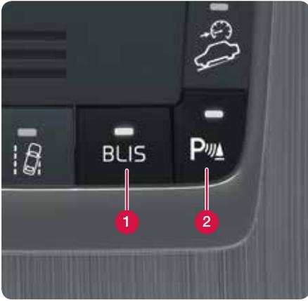
**Blind Spot Information System (BLIS)** indicates the presence of a fast approaching vehicle or a passing vehicle in the door mirror's blind area.
