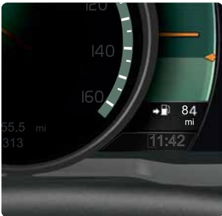
This is the approximate distance that can be driven on the remaining fuel based on average fuel consumption during the last 20 miles (30 km) of driving (digital\* instrument panel shown).
