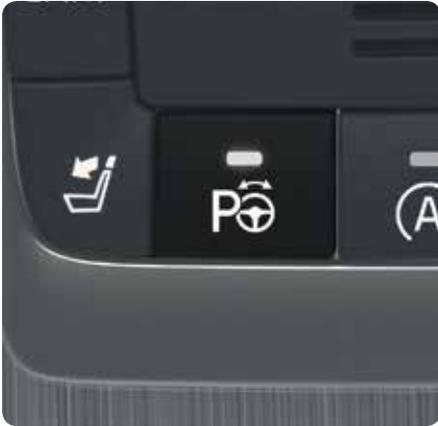
PAP determines if a parking space is big enough for your vehicle and helps to steer it into the space. The driver selects gears, regulates the vehicle's speed and applies the brakes.
