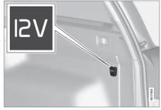
Fold down the cover to access the electrical socket. It works even when the remote control key is not in the ignition switch.
