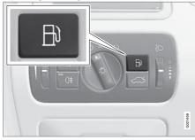
Open the fuel filler flap using the button on the lighting panel. The filler flap is located on the right-hand rear wing, as indicated by the sym-
