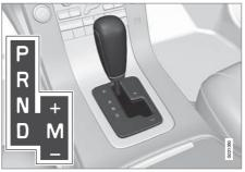
The information display shows the position of the gear selector using the following indications: P, R, N, D, S, 1, 2, 3, 4, 5 or 6, see page 65.
