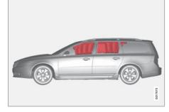
The inflatable curtain (IC) is a supplement to the SIPS and SRS airbags. It is fitted in the headlining along both sides of the roof and protects the car occupants sitting in the outer seats. A sufficiently violent collision trips the sensors and the inflatable curtain is inflated. The inflatable curtain helps to prevent the driver and passengers from striking their heads on the inside of the car during a collision.
