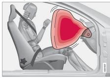
The car has an airbag to supplement the protection afforded by the seatbelt on the passenger side. This airbag is folded up into a compartment above the glovebox. Its cover panel is marked **SRS AIRBAG**.
