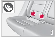
Mounting points for the ISOFIX fixture system are concealed behind the lower section of the rear seat backrest, in the outer seats.
