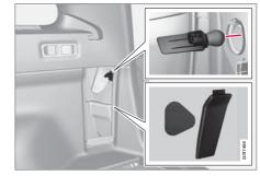
The direction indictor bulb in the rear lamp cluster is replaced from inside the cargo area.
