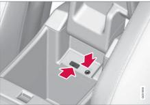
An iPod® or MP3 player can be connected to the car's infotainment system via the USB connection\* or AUX input in the centre console.
