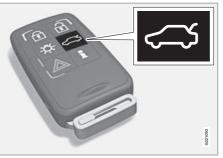
**Unlocking with the remote control key** The alarm for the tailgate can be disarmed<sup>\*</sup>, and the tailgate unlocked and opened on its own<sup>\*</sup> by using the remote control key.
