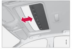
One long press on the lock button closes the sunroof and all the windows, see pages 41 and 50. The doors and the tailgate are locked. To interrupt closing, press the lock button again.
