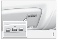
HomeLink<sup>®</sup> is a programmable remote control which can control up to three different devices (e.g. garage door, alarm system, outdoor lighting and indoor lighting etc.) and in doing so replace their remote controls. HomeLink is supplied built into the left-hand sun visor.
