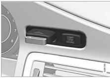
Ignition switch with inserted remote control key.
