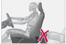
Do not leave any objects on the floor behind the driver's seat or the passenger seat.
