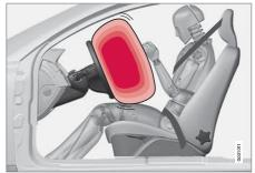
The car has an SRS airbag (Supplemental Restraint System) to supplement the protection afforded by the seatbelt on the driver's side. This airbag is fitted into the centre of the steering wheel. The steering wheel is marked **SRS AIRBAG**.
