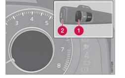
1 Thumbwheel. Turn the rotary control until the display shows **Driver**
