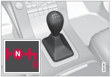
The reverse gear inhibitor hinders the possibility of mistakenly attempting to engage reverse gear during normal forward travel.
