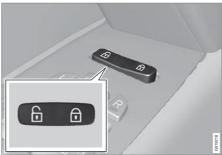
All of the doors and the tailgate can be locked or unlocked simultaneously using the central locking button on either front door. Press one side  $\fbox{1}$  of the button to lock - the other side  $\fbox{1}$  to unlock.
