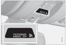
Indicator in the roof console showing that the passenger airbag is deactivated.
