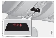
Unbelted occupants will be reminded to fasten their seatbelts by means of an audio and visual reminder. The audio reminder is speed dependent, and in some cases time dependent. The visual reminder is located in the roof console and the combined instrument panel.
