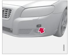
Electrical input to the engine block heater.
