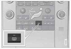
Use the defroster to quickly remove misting and ice from the rear window and the door mirrors.
