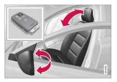
When the car is unlocked with the same remote control key and the driver's door is opened the driver's seat and also the door mirrors automatically adopt the positions stored in the key memory.
