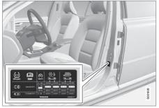
The tyre pressure label on the driver's side door pillar (between front and rear door) shows which pressures the tyres should have at different loads and speed conditions, this is also specified in the tyre pressure table, see below.
