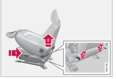
The passenger seat backrest can be folded forward to make room for long loads.
