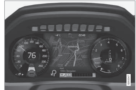
The instrument panel displays information such as speed, an incoming phone call or the track
