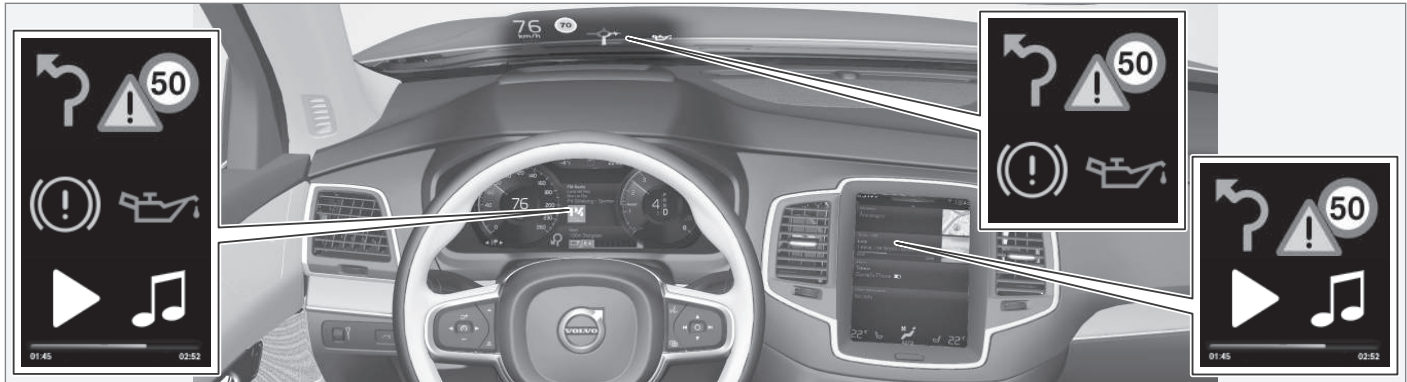
Information is presented in different displays depending on how it should be prioritized (generic illustration)
