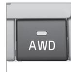
Use this button on the centre console to activate all-wheel drive (AWD - All Wheel Drive), see Drive system - drive modes (p. 268). The mode is primarily intended for use at low speed in slippery driving conditions.
