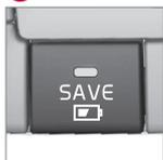
This function starts charging the hybrid battery and ensures that its energy level does not fall below a capacity equivalent to approx. 20 km driving with electric operation. The idea is to be able to save this energy
