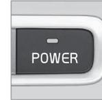
This option sets the car in the best response and performance mode, by means of both the electric motor and fuel-driven engine being activated the whole time. The car has sportier characteristics and faster response to accelerating.
