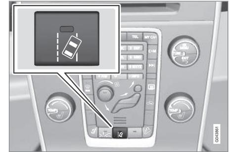
Press the centre console's button to activate or deactivate the function. The button's lamp illuminates when the function is switched on.
