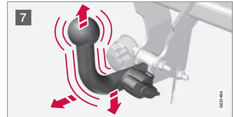
7 Check that the towbar is secure by pulling it up, down and back.
