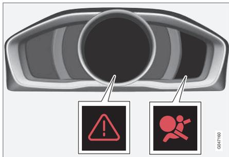
Warning triangle and warning symbol for the airbag system (p. 34) in the combined instrument panel.
