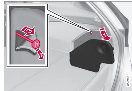
1. Open/remove the side hatch in the cargo area (same side as fuel filler flap).
