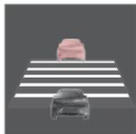
Only when the symbol shows an image of another vehicle is the **distance** to the vehicle in front controlled by the ACC.
