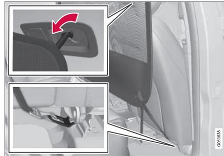
4. Hook the hook into the eyelet on the seat rail on both sides and tension the cam lock by pressing down the tongue and tensioning the strap.
