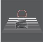
Different time intervals to the vehicle in front can be selected and shown in the combined instrument panel as 1-5 horizontal lines - the more lines the longer the time interval. One line corresponds to approximately 1 second to the vehicle in front, 5 lines approximately 3 seconds.
