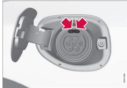
The LED lamps show the current status while charging is in progress. The white, blue, red and yellow lamps are activated when the passenger compartment lighting is switched on - they remain switched on for a while after the passenger compartment lighting has been switched off.
