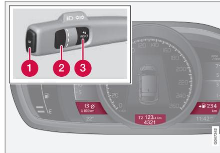
Three trip computer options can be displayed simultaneously - one in each "window".
