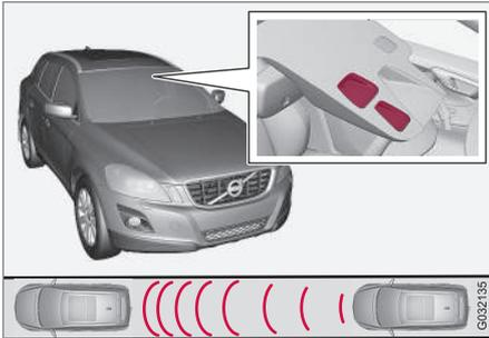
Laser sensor transmitter and receiver window<sup>10</sup>.
