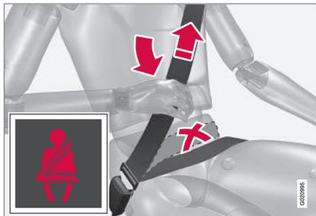
Tension the hip strap over the lap by pulling the diagonal shoulder belt up towards the shoulder. The hip strap must be positioned low down (not over the abdomen).
