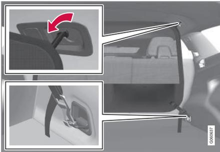
3. Hook the hook into the load retaining eyelets on both sides and tension the cam lock by pressing down the tongue and tensioning the strap.
