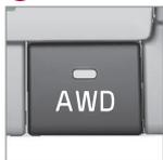
The mode activates all-wheel drive, which improves the car's grip and traction. The mode is primarily designed for low speed on slippery road surfaces, but all-wheel drive also has a stabilising effect at higher
