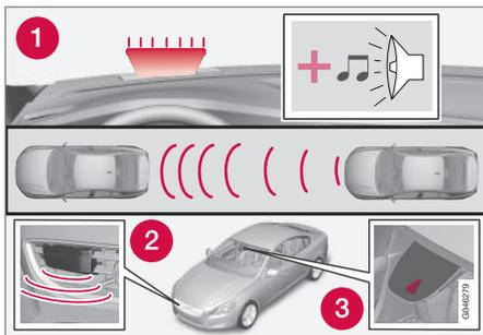
1. Collision warning system warning lamp and warning sound<sup>6</sup>.
