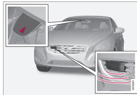
Camera and radar sensor<sup>18</sup>.
