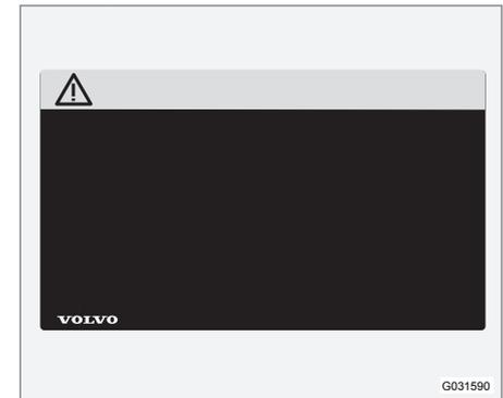
Black ISO symbols on yellow warning field, white text/image on black message field. Used to indicate the presence of danger which, if the warning
