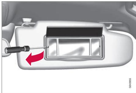
1. Insert a screwdriver under the lamp lens and gently prize up the lug on the edge.
