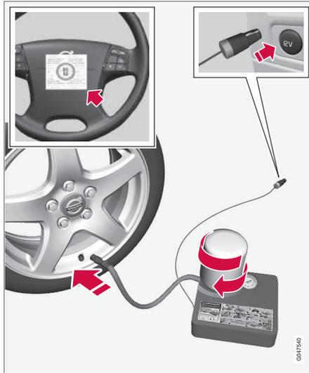
For information on the function of the parts, see Emergency puncture repair kit - overview (p. 345).
