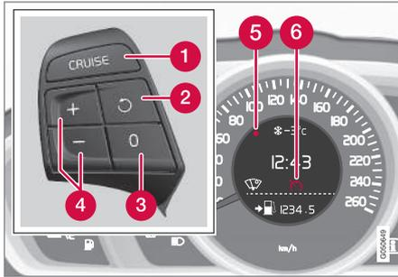
The steering wheel buttons and combined instrument panel in cars **without** speed limiter<sup>2</sup>.
