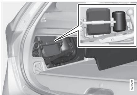
The lamps are accessible when emergency puncture repair kit is lifted out.
