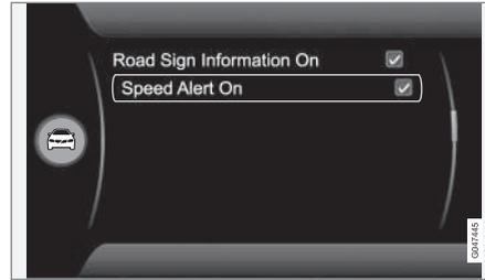
The driver can opt to receive a warning when the applicable speed limit is exceeded by 5 km/h (5 mph) or more. This warning is given by the symbol showing the applicable maximum speed temporarily flashing when this speed is exceeded. The function can be activated/deactivated in the menu system **MY CAR**. For a description of the menu system, see MY CAR (p. 115).
