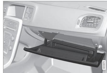
The owner's manual and maps can be kept in here for example. There are also holders for pens on the inside of the lid. The glovebox can be locked\* (p. 181) using the key blade (p. 169).
