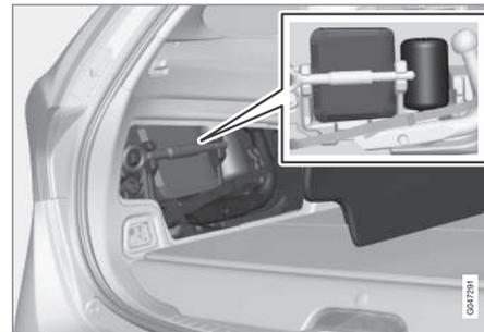
The puncture repair kit is behind the hatch on the left-hand side of the cargo area.
