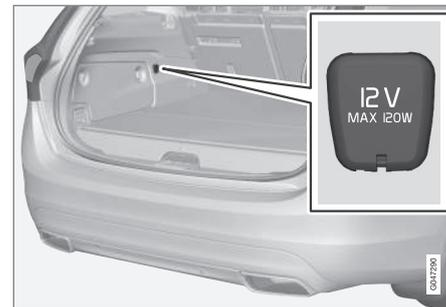
Lower the cover to access the electrical socket.
