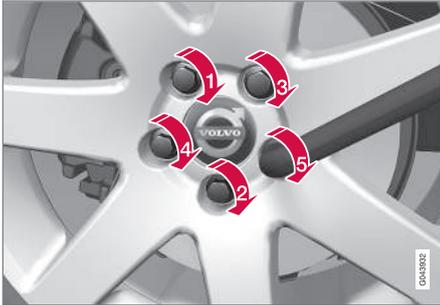
4. Tighten the wheel bolts crosswise. It is important that the wheel bolts are tightened properly. Tighten to 140 Nm. Check the torque with a torque wrench.
