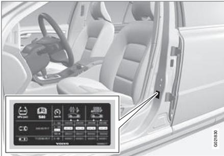
The tyre pressure label on the driver side's door pillar (between frame and rear door) shows the tyre pressures for the car's recommended tyre dimensions. This is also specified in the tyre pressure table, see Tyres - approved tyre pressures (p. 423).
