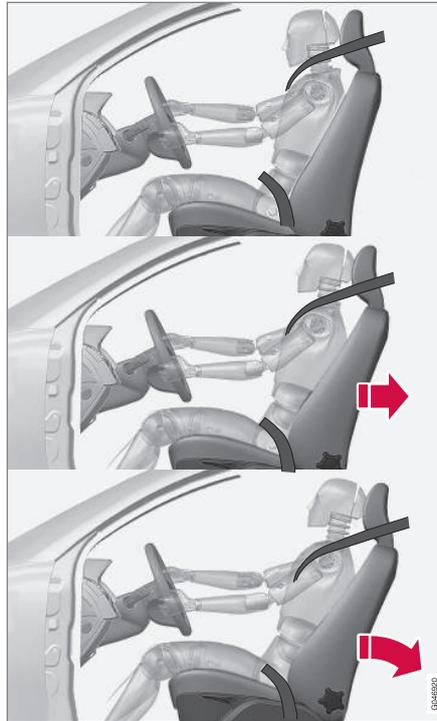
The WHIPS system is actuated by a rear-end collision, where the angle and speed of the collision,
