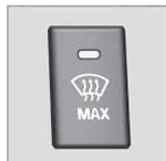
Air flowing to the windows. The light in the defroster button illuminates when the function is active.
