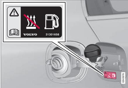
The fuel filler cap can be attached onto the flap.
