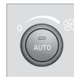
Turn the knob to increase or decrease fan speed. If **AUTO** is selected, then the fan speed is regulated automatically (p. 133) - the fan speed previously set is disengaged.
