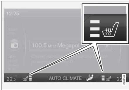
Current heat level is shown in the centre console display screen.
