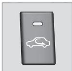
When recirculation is engaged the orange lamp in the button illuminates.
