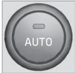
If you select one or more manual functions, the other functions continue to be controlled automatically. All manual settings are disengaged when **AUTO** is pressed. The display screen shows **AUTO**
