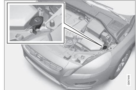
Topping up the washer fluid takes place by opening the blue cap.
