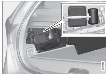
The car's towing eye, emergency puncture repair kit and the tool for the plastic wheel bolt caps are located behind the hatch on the left-hand side of the cargo area. There is also space for the sleeve for the lockable wheel bolts. Jack\* and wheel wrench\* are located in a bag on the cargo area floor.
