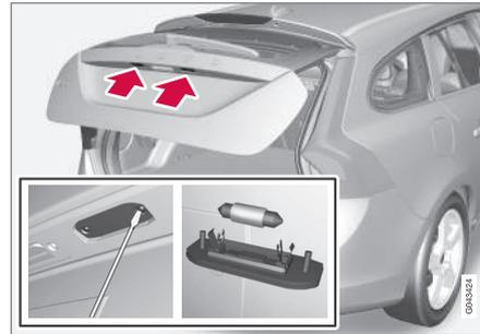
1. Remove the screws with a screwdriver.
