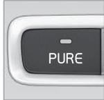
This option focuses on electric operation as well as low energy consumption, and helps the driver to maximise driving on the hybrid battery.
