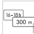
Some speeds are applicable only after e.g. a specific distance or at a certain time of day. The driver's attention is drawn to the situation by means of a symbol for an additional sign under the symbol showing speed.
