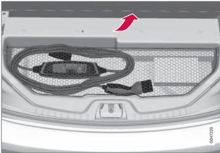
The charging cable is located in the storage compartment under the cargo area's floor cover.
