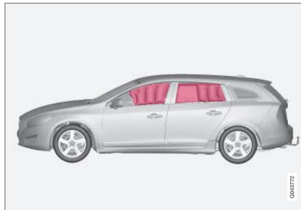
Inflatable curtain IC (Inflatable Curtain) is part of the SIPS system (p. 39) and the airbag system (p. 34). It is fitted along both sides of the headlining and helps protect the driver and passengers in the car's outer seats. A sufficiently violent collision trips the sensors and the inflatable curtain is inflated.
