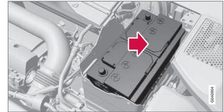
1. Lower the battery into the battery box.
