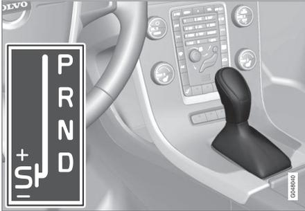
**D:** Automatic gear positions. **+/-:** Manual gear positions.
