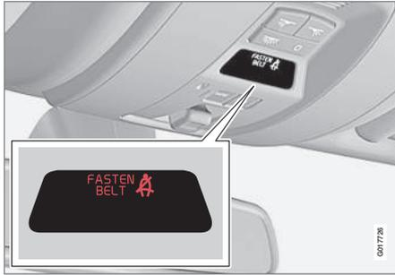
The audio reminder is speed dependent, and in some cases time dependent. The visual reminder is located in the roof console and in the combined instrument panel (p. 68).
