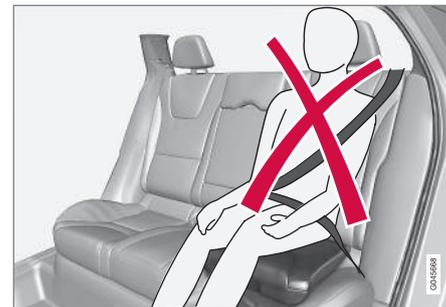
Incorrect positioning, the seatbelt must not be placed beneath the shoulder.
