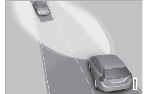
Adaptive functionality: Dipped beam directly toward oncoming vehicles, but continued main beam on both sides of the vehicle.
