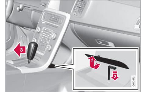
If the car cannot be driven, e.g. due to a flat starter battery, the gear selector must be moved from the **P** position so that the car can be moved.
