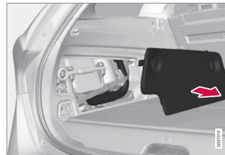
3. Take out the jack\*, tool to remove the plastic caps on the wheel bolts and the wheel wrench\* (located in a bag on the cargo area floor). If another jack is selected, see Raising the car (p. 355).
