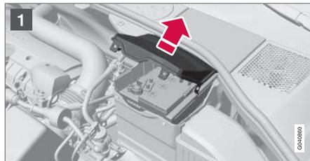
5. Open the clips on the front cover of the battery in your car **1** and remove the cover.
